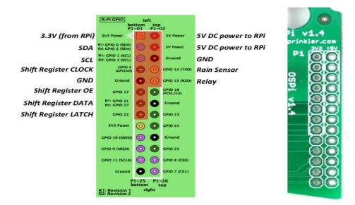
corner of the circuit board. The layout of the mapped out pins match the GPIO pins. Pins use by OSPi is marked by a white outline.
